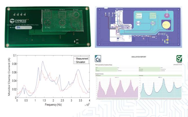
"Simyog's Compliance-scope was used to analyze the Bulk Current Injection on a product design. We could clearly observe how the impedance mismatch in one of the differential lines which eventually led to common mode currents and errors in data frames sent on these differential lines. Compliance scope can be used by any hardware engineer to easily arrive at a conclusion at an early stage."
